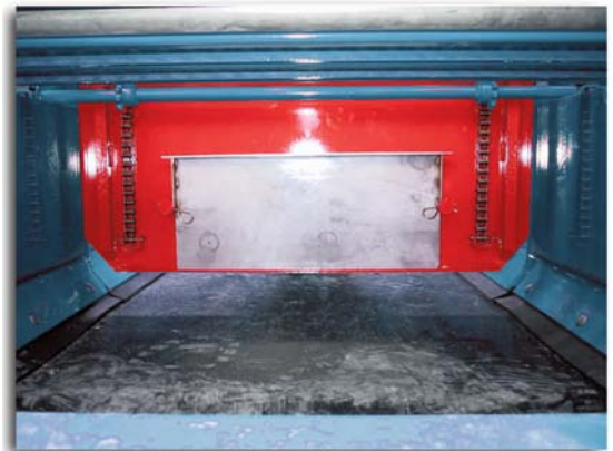
GUILLOTINE SHUTTER IN REST POSITION
