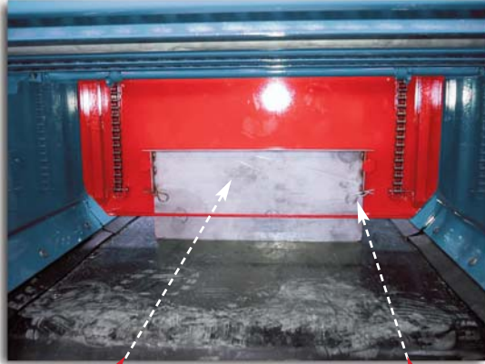
GUILLOTINE SHUTTER IN WORKING POSITION
